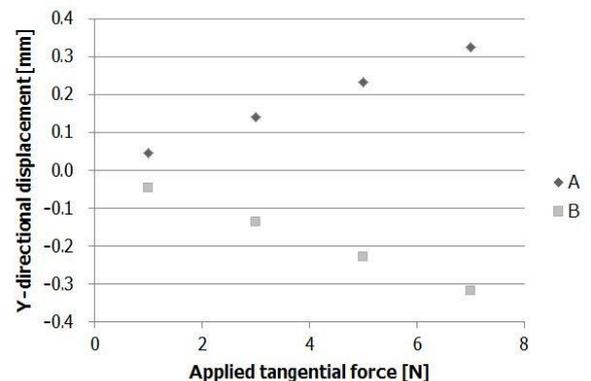
Figure 5. Y-directional displacement with tangential force at the measurement points A and B.
