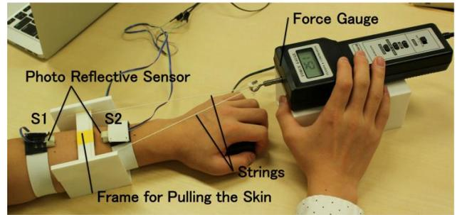
Figure 7. Experimental tool for applying tangential force in a step-by-step manner. Digital force gauge measures pulling force.
