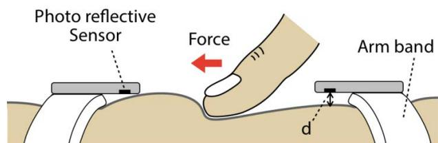
Figure 2. Armband type sensor that enables to measure tangential force given to skin surface.
