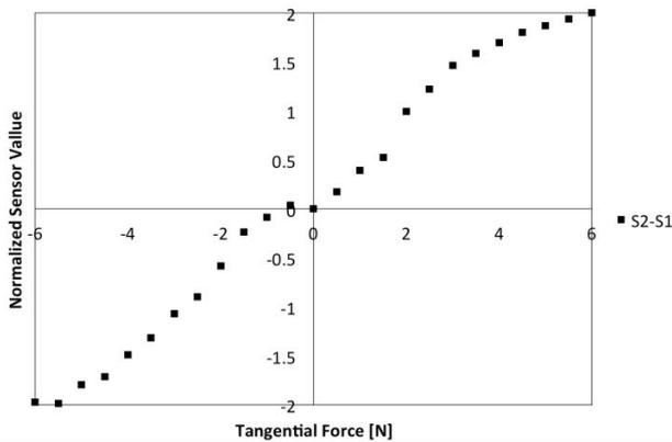
**Figure 9. Difference between normalized S1 and normalized S2 against tangential force of skin.**
