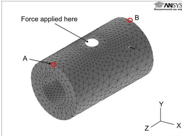
Figure 3. FEM simulation model.
