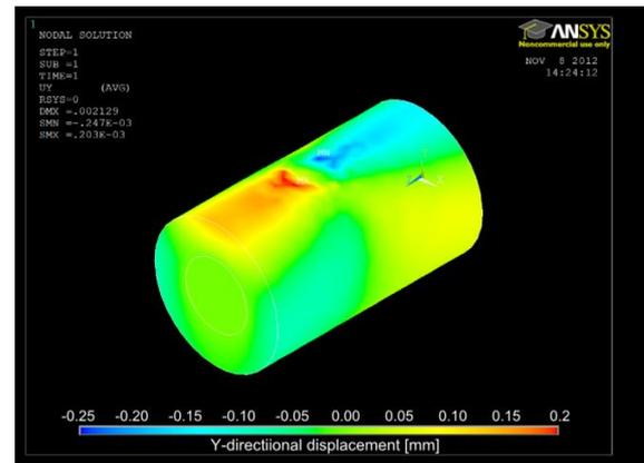
Figure 4. Simulation result of y-directional displacement with 3 N tangential force.
