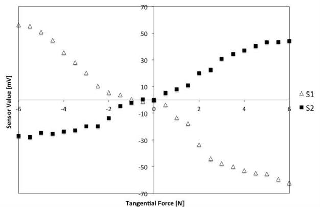
Figure 8. Average measured voltage against tangential force of skin.
