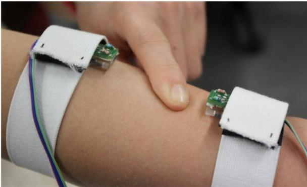
Figure 1. The belt type sensor that enables to measure the tangential force generated onto skin surface.
