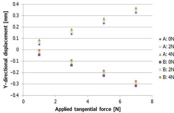
Figure 6. Y-directional displacement with tangential force by changing the offset normal force.
