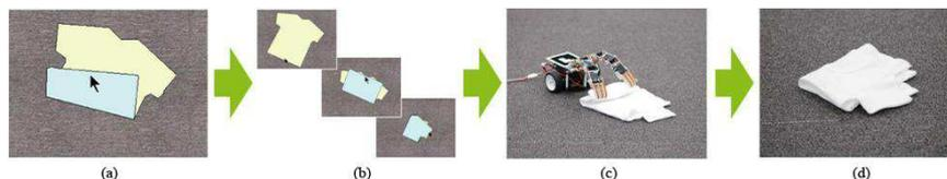
**Figure 1:** Teaching how to fold a T-shirt by means of graphical editing. The user folds the T-shirt on the computer via simple dragging operations (a, b). The robot then performs the task in the real world (c, d).
